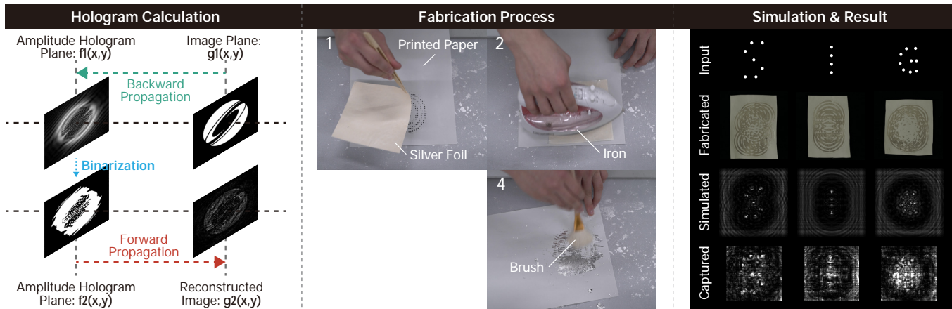
Figure 2: Left: designing an amplitude-modulated hologram. Center: fabrication flow. Right: results of our method (SIG letter).
