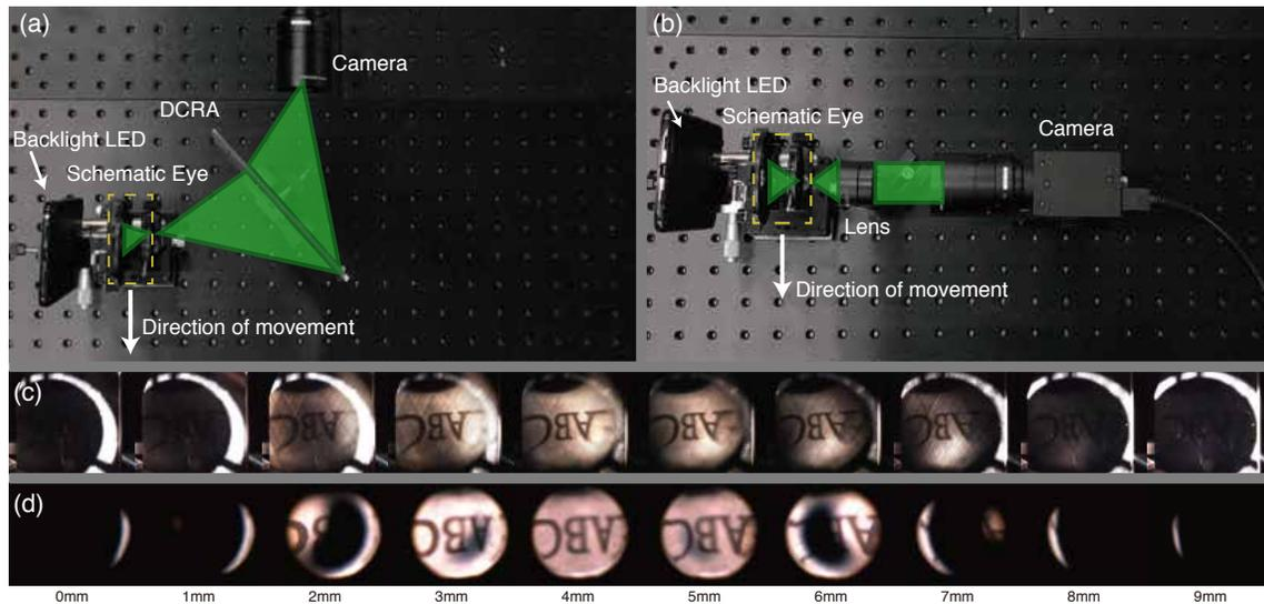
**Figure 2: Comparison of the optical system and eyebox measurement. (a) The proposed method using a DCRA. (b) Conventional system based on a Maxwellian view. (c) Captured images by the proposed method. The eyebox is 8 mm. (d) Captured images by conventional method. The eyebox is 3 mm.**
