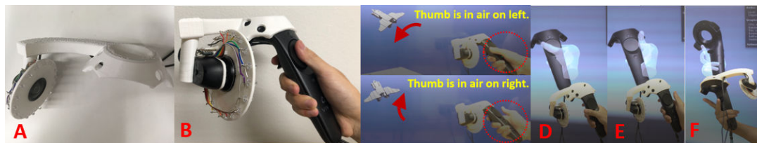
Figure 1: (A) Our prototype includes a NIR camera sensor. (B) While holding the Vive controller, the system is used to predict finger postures in real-time. EXController provides extra input from finger postures that can interact with VR content. (C) is an application that provides thumb postures in air to control an object's movements in the air. We developed a real-time Unity demo that maps the postures to matched finger animations (D, E, F), which is able to enhance "hand presence" while holding the controller.
