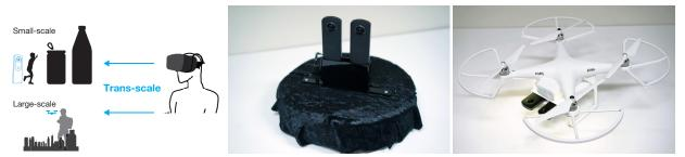
Figure 1. Left: Concept of a small-scale to large-scale trans-scale telexistence system. Middle: Our small-scale telexistence system comprising a controllable robot and omnidirectional cameras. Right: Our large-scale telexistence system comprising a drone.
