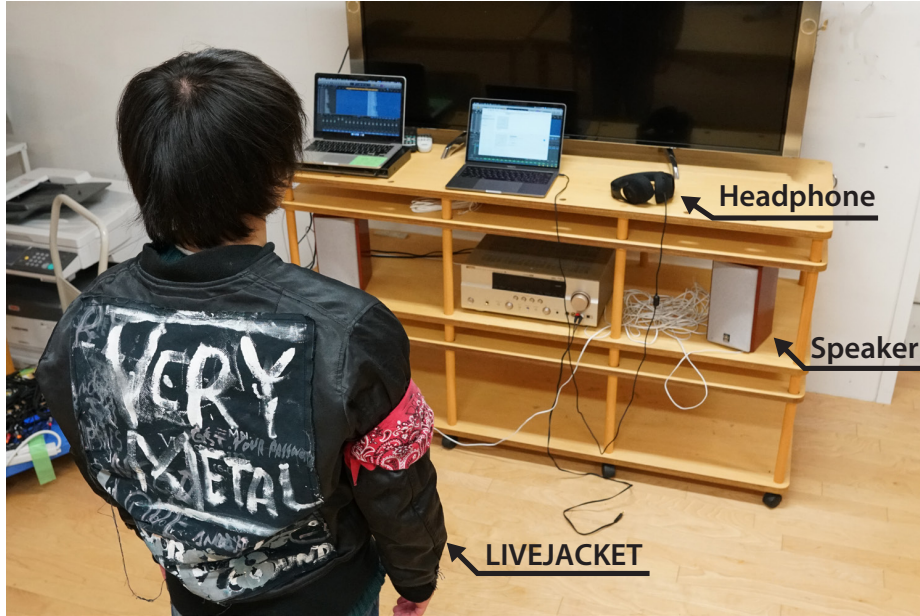
Fig. 3. Experiment setup. Subjects wore the LIVEJACKET and listened to music while standing.
