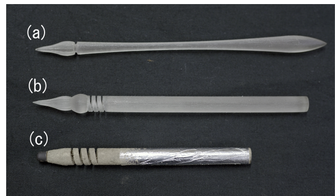
Figure 2: Development of three types of pens using 3D printers. (a) Glass dip pen. (b) Our proposed pen. (c) Spring pen.
