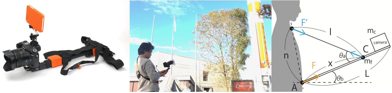
Figure 1: Left: our instrument assembly. Some parts consist of ready-made goods and components printed with a 3D printer. Center: an example of a shooting situation using our instrument. Right: simple configuration of our instrument. This image includes the applied forces, the masses of a few components, and the angles when the user is equipped with our instrument.
