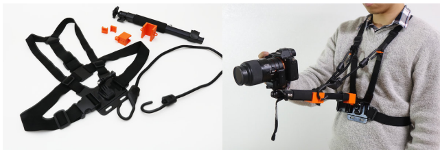
Figure 2: Left: all parts we prepared, consisting of a monopod, harness, bungee code, and 3D-printed components. Right: the user equipped with our instrument. The monopod is equipped with a movable panhead, therefore users can move a camera attached to the panhead freely.
