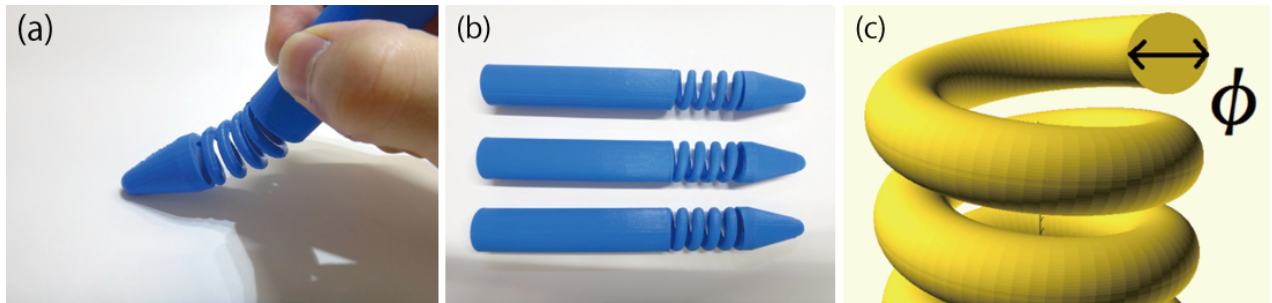
Figure 1: (a) Spring-Pen prototype model (not conductive filament). (b) \phi=4.5\text{mm}, 5.0\text{mm}, 5.5\text{mm} . (c) Coil spring diameter \phi .
