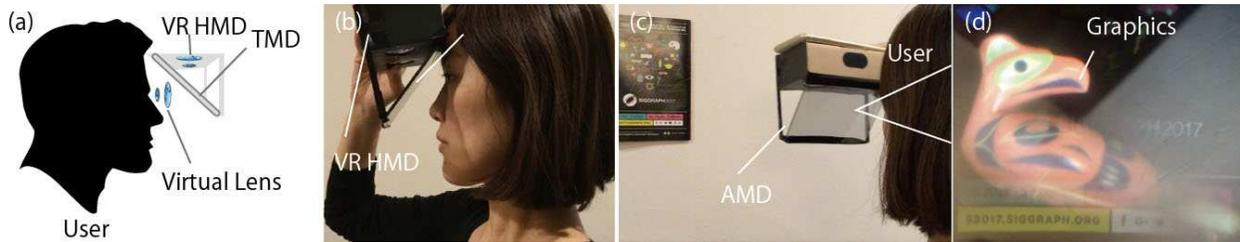
Figure 8: Application of see-through wide view angle HMD. (a) System layout. (b) Setup. (c), (d) Obtained image with aerial image and background scene.
