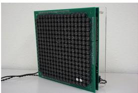
**Figure 4:** Ultrasonic-phased array.
