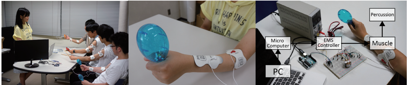
Figure 1: Left: participants having a combined session with our system. Middle: EMS signal stimulates the muscle, the user's arm reacts, and generates percussive sound from held maracas. Right: overview of our system.
