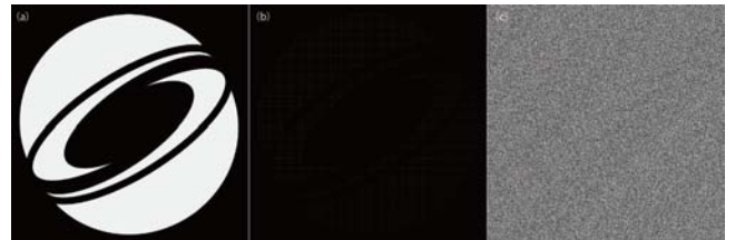
Figure 5: Example of a computer-generated hologram (CGH). (a) An original image, (b) a converted spot-array image of the original image, and (c) a CGH to be displayed on the SLM.
