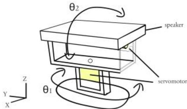
Figure 3. Structure of two axis servo direction controller we used.
