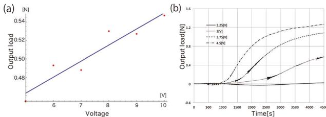
**Figure 3:** (a) Output load of SMA varies according to applying voltage. (b) Response speed of Coded Skeleton varies according to applying voltage.
