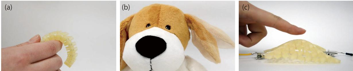
**Figure 1:** Application example of Coded Skeleton. (a) Shape memory application. (b) Deformable skeleton. (c) Actuated button.
