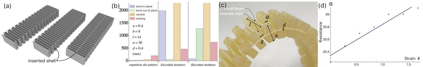
**Figure 2:** (a) The structures of Coded Skeleton: repetitive slit pattern, (A) Coded Skeleton and (B) Coded skeleton. (b) Eigenmode and eigenvalue of Coded Skeleton. (c) Ruling line and structural parameters of Coded Skeleton. (d) Strain and resistance of coded skeleton
