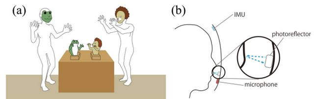
Figure 2: (a) System image of Yadori. (b) Design inside our mask-type device.
